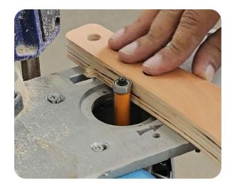
2. Clean the tabs off. The fastest way to do this is to use a router table with a flush trim bit that has a bearing.
