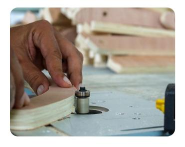
3.2 Clean the tabs off. The fastest way to do this is to use a router table with a flush trim bit that has a bearing.
