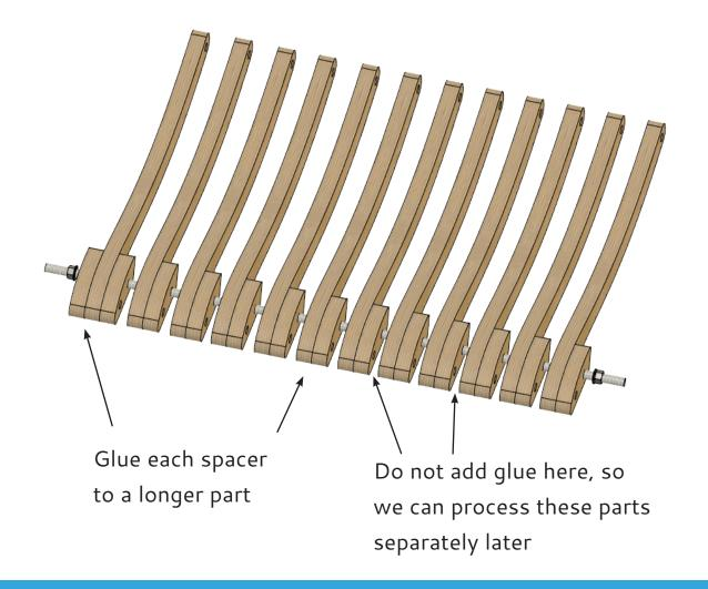
6.3 Add another threaded rod to make sure all the parts are aligned properly
