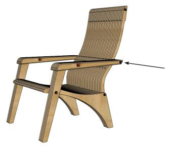
11.6 Insert the last rod here to attach the arm rests to the back rest
