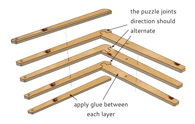
4.6 Clamp the parts or use brad nails to hold the layers tight while the glue is drying
