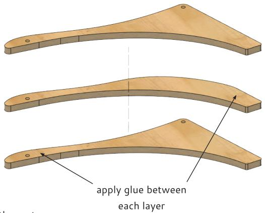
5.3 Clamp the parts or use brad nails to hold the layers tight while the glue is drying
