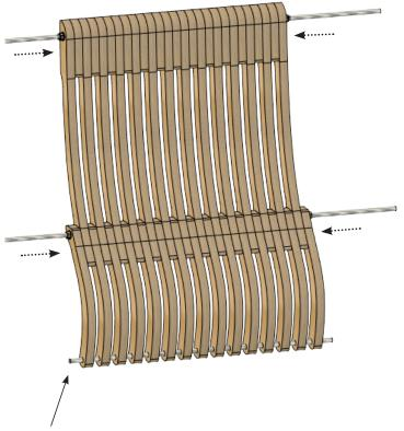
7.4 Add another threaded rod to make sure all the parts are aligned7.5 Align all the layers and tighten the nuts to clamp all the layers together
