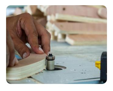
3.2 Clean the tabs off. The fastest way to do this is to use a router table with a flush trim bit that has a bearing.
