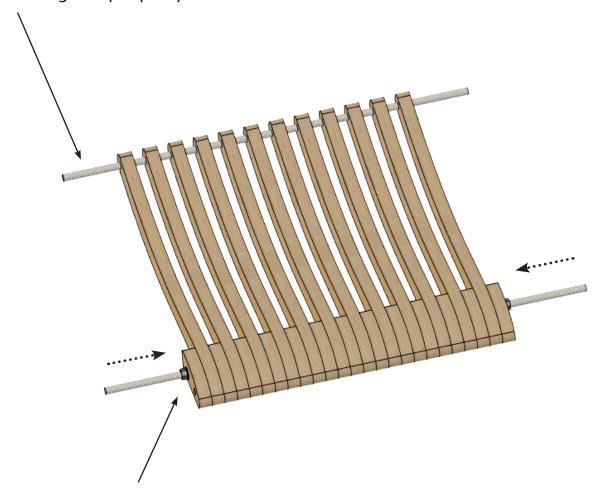
6.4 Align all the parts and tighten the nuts to clamp all the parts together6.5 Leave over night to dry
