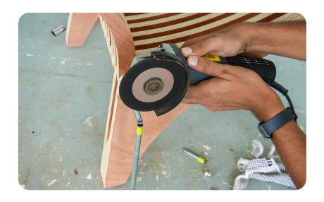
12.2 Take the rods slightly out and cut them to final length with a hack saw or a grinder
