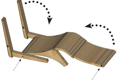
11.5 Add a rod in the top of the back rest and lift it
